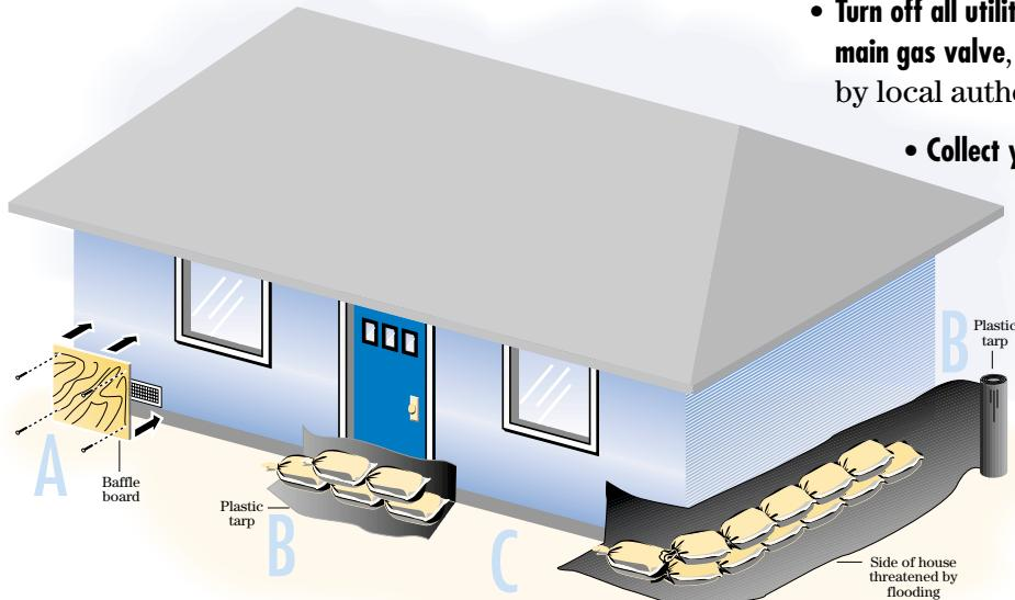
**A** **Baffle boards** consist of 3/4 inch plywood sheets with a soft gasket material like felt or foam rubber. They are effective for closing off vents, low windows and doors from floodwater. If placed over vents, however, baffle boards must be removed once the danger of flooding passes.
