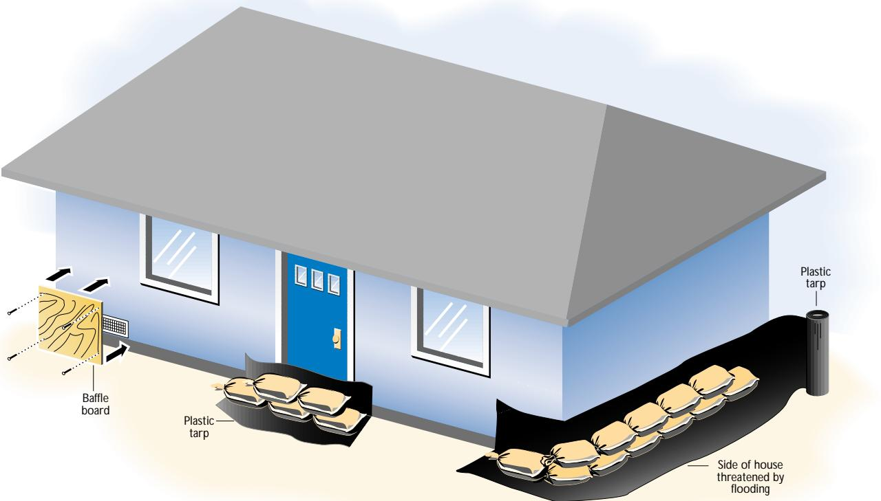
Baffle boards (above left) consist of 3/4 inch plywood sheets with a soft gasket material like felt or foam rubber. They are effective for closing off vents, low windows and doors from floodwater. If placed over vents, however, baffle boards must be removed once the danger of flooding passes.
